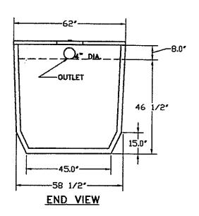
TANK: CATEGORY 3. 2.5" 900 GALLON 2 COMPARTMENT TANK REINFORCED WITH FIBRILLATED POLYPROPYLENE FIBER. 2.5" WALLS AND 3" BOTTOM. INLET AND OUTLET RESILIENT CONNECTORS PER ASTM-923-98. CONNECTORS MUST BE USED WITH APPROVED CLAMP. CONNECTOR WILL ACCEPT 4" PVC PIPE.
