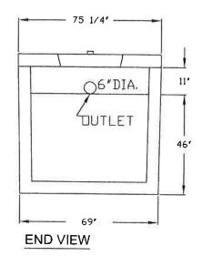
TANK: CATEGORY 4. 4" 1530 GALLON 1 COMPARTMENT TANK REINFORCED WITH #3 STEEL 12" O/C. BOTH WAYS. 4" WALLS AND 4" BOTTOM. INLET AND OUTLET RESILIENT CONNECTORS PER ASTM-923-98. CONNECTORS MUST BE USED WITH APPROVED CLAMP. CONNECTOR WILL ACCEPT 6" PVC PIPE.
