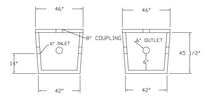
$\underline{\mathsf{TANK:}}$  8" SAMPLING BOX REINFORCED WITH #4 STEEL 6" O/C. BOTH WAYS. 8" WALLS AND 8" BOTTOM. INLET AND OUTLET RESILIENT CONNECTORS PER ASTM-923-98. CONNECTORS MUST BE USED WITH APPROVED CLAMP. CONNECTOR WILL ACCEPT 8" PVC PIPE.
